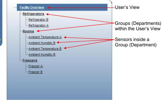
Any device monitored by TempTrak that you are in charge of is displayed in the Sensor list when you click the Sensor tab. Equipment is normally arranged into groups or departments, and all groups and departments are displayed in a user's view. Each line item can be clicked on and will provide additional detailed information.
