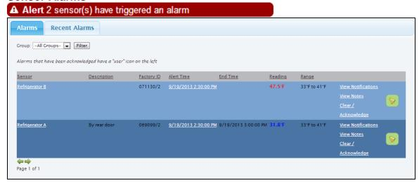
Sensor Alarms provides current information on the number of sensors with outstanding alarms that need to be addressed.
