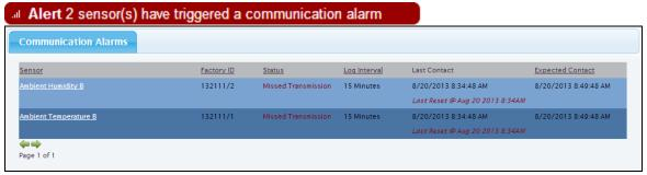
Communication Alarms shows which sensors are having difficulty communicating their information to TempTrak. Once the sensor starts communicating again, the communication alarm will be cleared.
